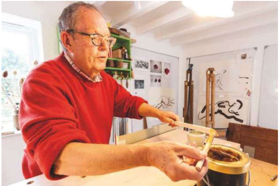
Stirring it up: One of the results of bringing in Chris Schwarz, David admits, is that, "I've been reminded about stuff I knew but had forgotten" – like the merits of hide glue for carcass work
